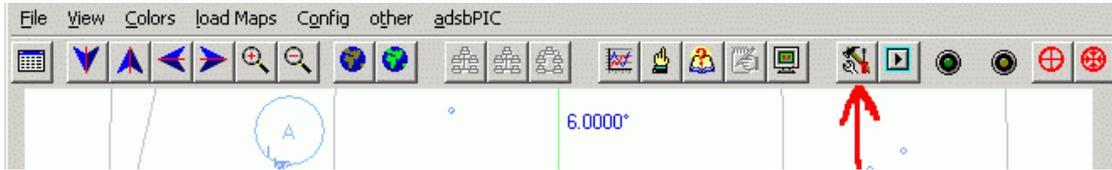
A little setup-window opens. Here you choose the correct com-port number for the attached decoder.
